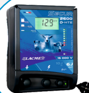
No. 201-010-018 SECUR 2600-D HTE mains energizer • max. length of the fence line: 55 km • peak voltage: 15 000 V • output energy: 6000 mJ • stored energy: 10 000 mJ • additional power output: 1200 mJ • digital display allows checking vegetation growth • immediate fence control by means of graphic indicators and accurate voltage display numbers • voltage test LED bar • adapted for response devices • lamp for return lead of electric fence
